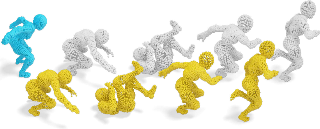
Figure 1. Non-rigid registration on 3D point sets. The blue and gray models represent the source and target point clouds, respectively, while the yellow models are our registration results. Our method achieves successful registrations even for shapes with challenging deformations.
